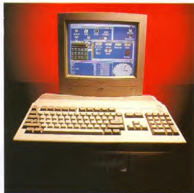
Having proved its appeal many times over since being released in the late Eighties, the A500 can be upgraded internally to nearly as good as an A500P. The main difference is that expansions which fit in the trap-door slot are not compatible between the two machines. If you're using one of these and you want a better Workbench, think about upgrading.
